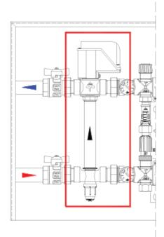
Composition of manifold kit with zone valve: **L1 + 110 mm**
