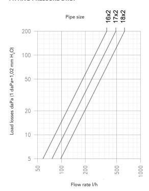
Pressure drop of a pair of fittings for PE pipes. (Not to be considered for annealed copper pipes. The fittings used for these pipes do not generate significant pressure drops).
